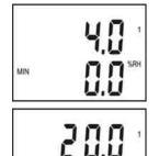
Range and type of value for output 1 (current loop I1 = symbol ,,1"on display). Type of value, assigned to output 1, is indicated by displayed unit (here %RH = relative humidity). Upper line displays current value corresponding to measured value (lower line).
