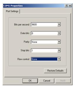
• Select item "File", "Features" in menu. Select bookmark "Setup", in the window, click on "ASCII Setup… " and modify all items in accordance with following figure and press OK
